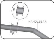
Corret position of the parts "F" on handlebar 28 mm, 1.102 inch.
